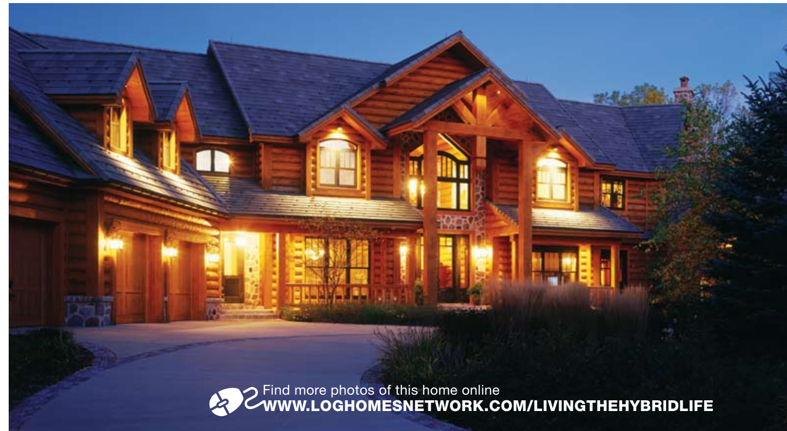
Left: The hybrid home features 12-inch handcrafted half-logs with a combination of saddle-notch and beam corners, timbers, and cut stone. The entrance showcases a custom door with sidelights and pentagonal window configuration flanked by a porch. A heated three-car garage, state-of-the-art security system, and steel front gate ensure more comfort. Below: Designed to take advantage of the waterfront view from the second floor, the loft game room features a sunken bar with comfy black leather chairs. Cowboy silhouettes are positioned in the custom triangle window above the French doors that open to the loggia.
